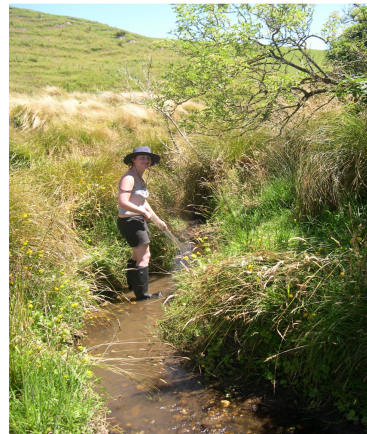
Figure 1. Sampling water quality and stream conditions on one of the ARGOS sheep/beef farms. Suzanne holds the water clarity tube, used to measure the amount of sediment in the water. This stream has an excellent buffer zone of dense vegetation to help prevent nutrients and sediment getting in to the water, but lacks shading, a potentially important screen that keeps water cooler and allows more fish to survive in the stream.
