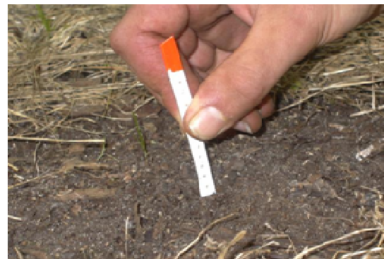
Figure 1: Bait-lamina probes used for assessing biological activity in the soil of kiwifruit orchards.
